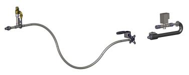
Add-on kit for LN2 multi mode cooling system 0CC30060B10.000-00 to fill the cooling agent tank without having to dismount the supply system, includes LN2 magnetic valve (for mounting into the supply system), connection tube (1.6 m long) to the storage tank (maximum operation over pressure 1.5 bar), handle with start button and safety valve.
