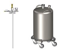
LN2 cooler, compressed gas (N2) operated supply system, with software-controlled magnetic valve, operating overpressure 0.5 bar, with cooling agent storage tank, made from stainless steel, content 60 l, with four mounted castors ø100 mm and carrying handles.
